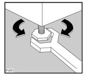
Any necessary adjustment can be made with a spanner. Accurate levelling prevents vibration, noise and displacement of the machine during operation.
